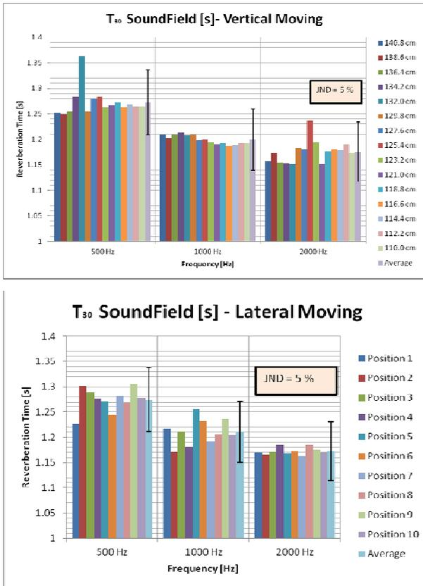
Figure 7: graphics about variability of parameter T30 for lateral and vertical moving at frequencies 500 Hz, 1000 Hz and 2000 Hz.
