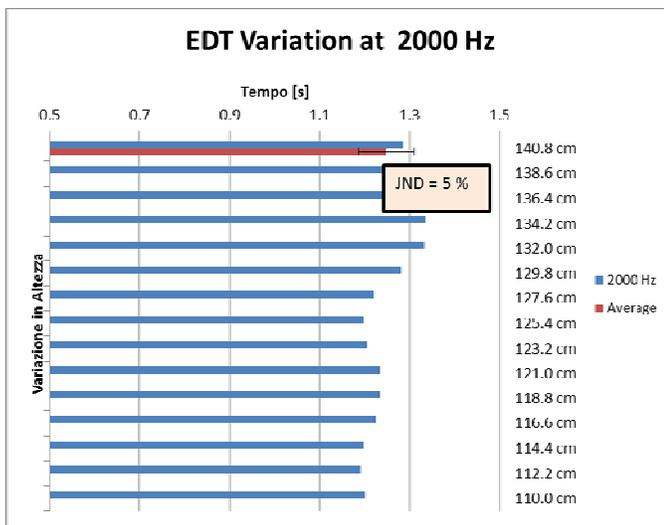
**Figure 4:** variability of parameter Early Decay Time (EDT) in vertical moving at frequencies from 125Hz to 8 kHz SoundField microphone
