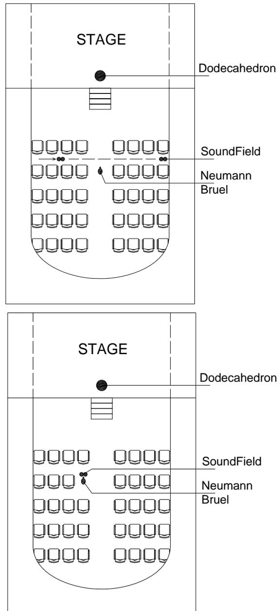
**Figure 2:** plans of Teatro 1763 Villa Mazzacorati, with positions of microphones for two type of measurements
