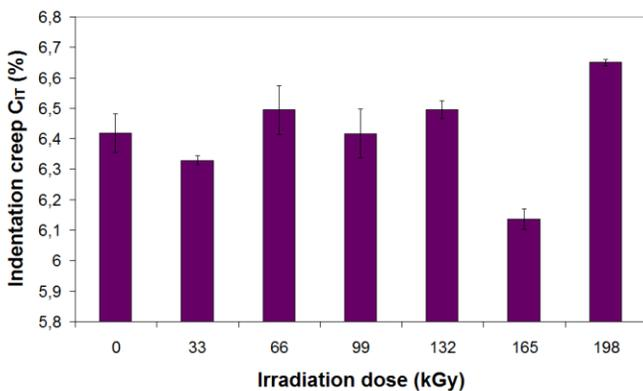
Fig. 6 Indentation creep of PC vs. irradiation doses
