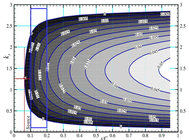
**Fig.8:** Contours of cross-flow disturbance spatial growth rates  $-\alpha_1\delta_{0.95}$  in supersonic swept wing BL for stationary disturbances in the plane  $(s/C, k_r)$ .
