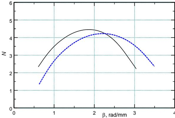
**Fig.14:**  $N$ -factors of stationary ( $\omega = 0$ ) cross-flow instability modes versus spanwise wavenumber, ( $s/C = 0.5$ ): local self-similar solution (solid line) and full boundary layer solution (dashed line).
