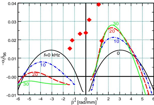
**Fig.12:** Spatial growth rates versus  $\beta^*$  [rad/mm], ( $s = 30$  mm). Symbols – experimental data [10] at  $f = 10$  kHz.
