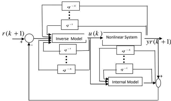
Fig. 3. Adaptive Internal Model Control (AIMC)
