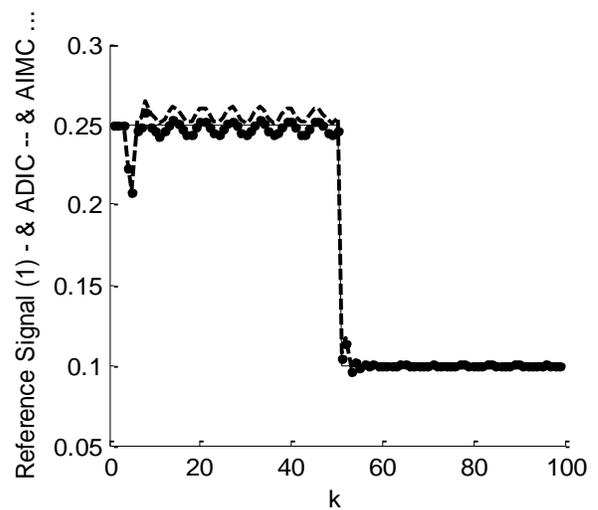
Fig. 7- The Output System using the ADIC, the AIMC and the Reference Signal (1)
