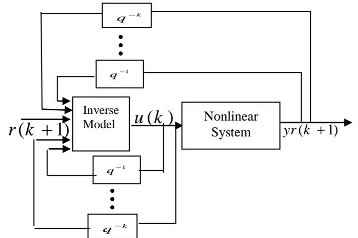
Fig. 2. The Adaptive Direct Inverse Control (ADIC)
