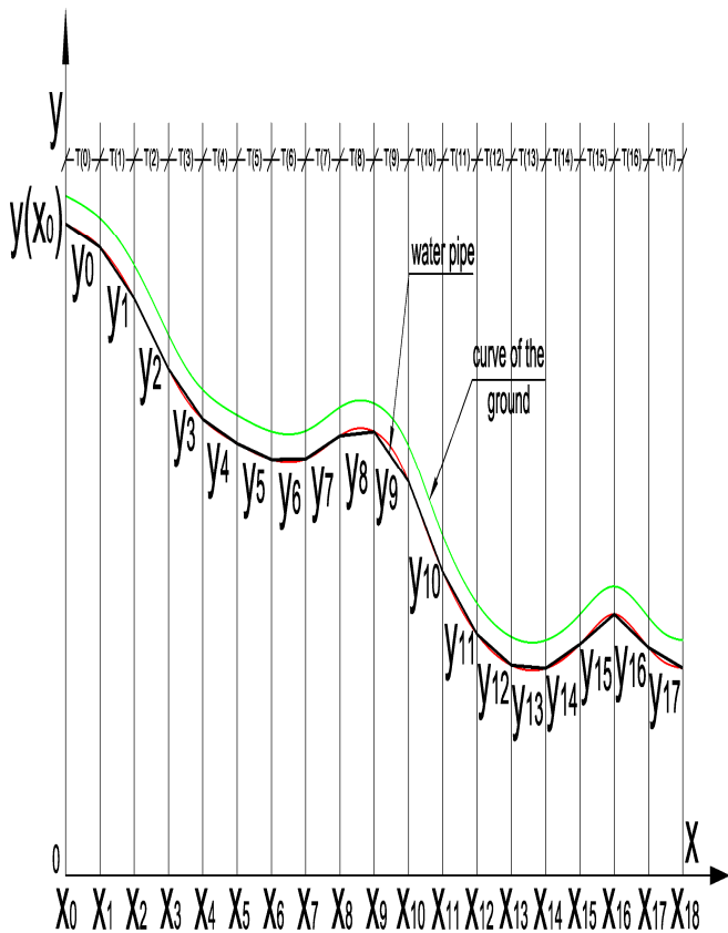
Fig. 4: represents an example of the MSF function (in black color) and the surface of the earth (in green color) and the optimal depth needed (in the red color).
