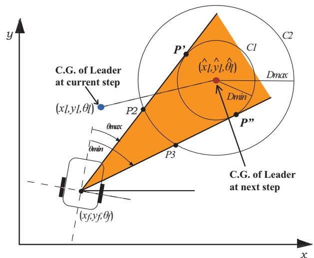
Fig. 7. The region restricted by angular velocity constraint
