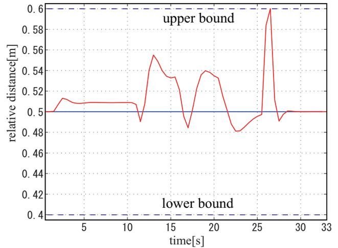
Fig. 13. Time fluctuation of relative distance with perturbation of  $l$  and  $c$  [ robust result (worst case) ]
