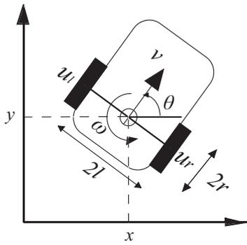
Fig. 1. Two-wheeled robot
