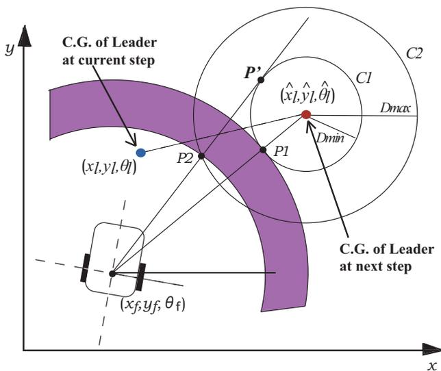
Fig. 6. The region restricted by velocity constraint
