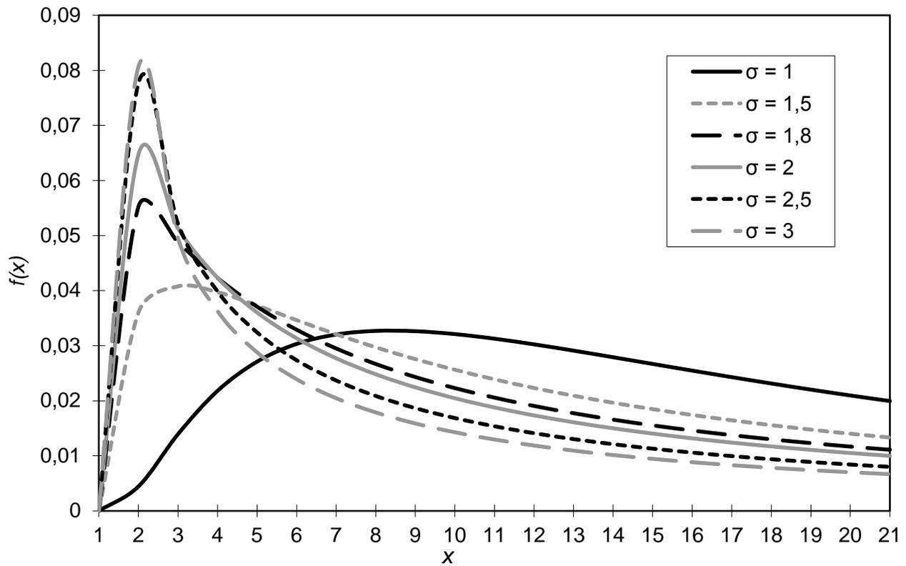
Fig. 3 Probability density function of two-parameter lognormal distribution for the parameter value  $\mu = 3$
