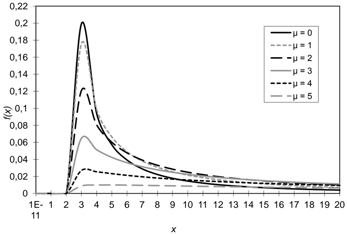
Fig. 4 Probability density function of three-parameter lognormal distribution for parameter values  $\sigma = 2$  ( $\sigma^2 = 4$ );  $\theta = 2$
