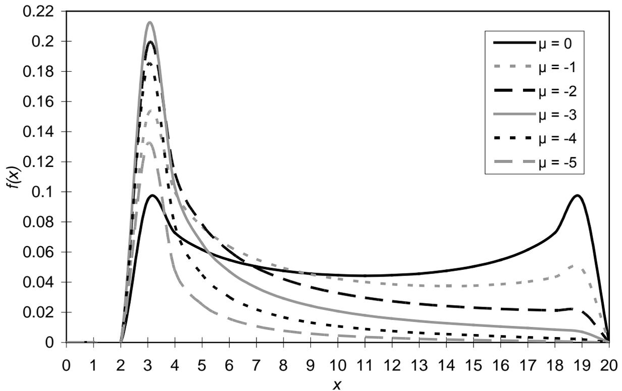
Fig. 7 Probability density function of four-parameter lognormal distribution for parameter values  $\sigma = 2$  ( $\sigma^2 = 4$ );  $\theta = 2$ ;  $\tau = 20$
