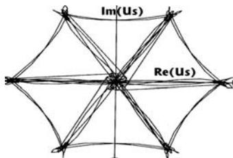
Fig.7 Fourier series approximation of the voltage space vector
