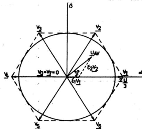
Fig.1 Voltage space-vector representation in  $\alpha\beta$  complex plane
