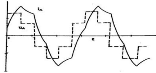
Fig.6 Six-step voltage and current waveform
