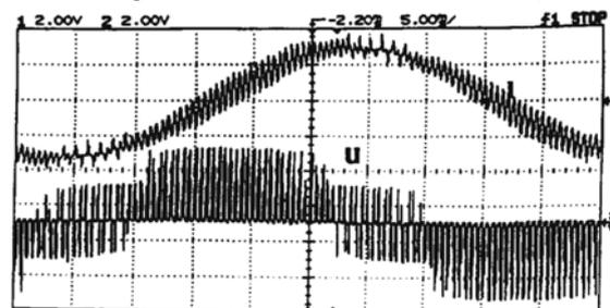
Fig.8 Experimental waveform of the stator voltage and current in phase
