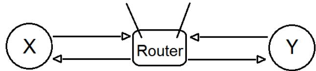
Fig. 1 A simple example demonstrating the throughput gain of using Network Coding
