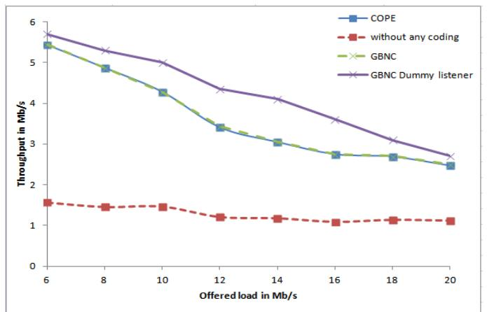
Fig. 4 Throughput gain against flow rate for unicast case
