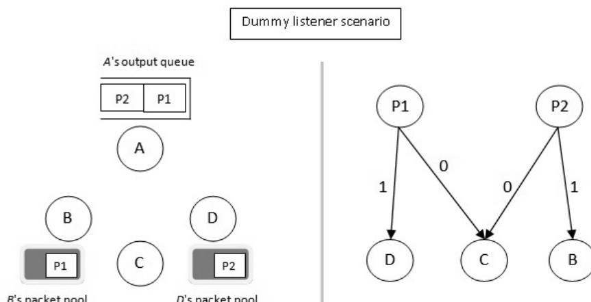
Fig. 3 A simple topology example with its equivalent graph representation
