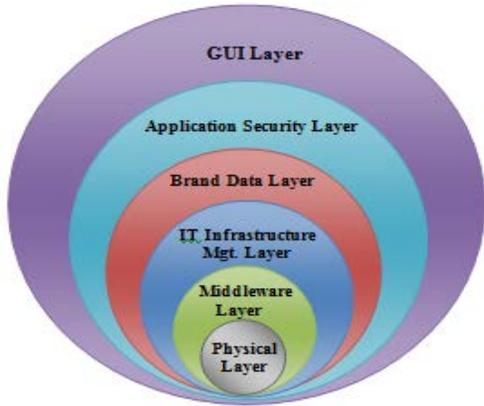
Fig. 3 multi-layer architecture for anti-counterfeit RFID systems
