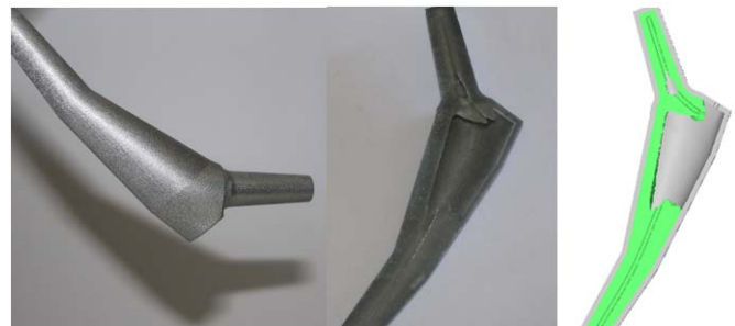
Figure 6 : optimization example for additive manufacturing
