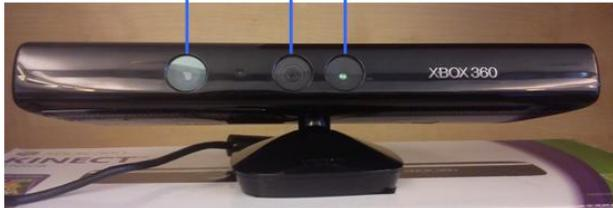
Fig. 1 Colour (RGB) and depth sensors in Kinect
