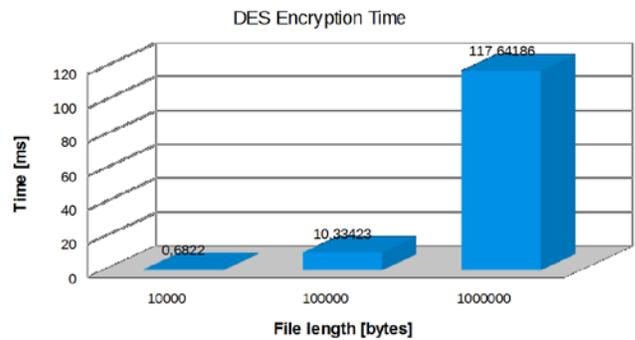
Fig. 17 DES Encryption time
