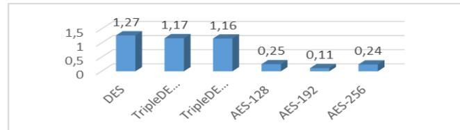
Fig. 31 average client CPU load
