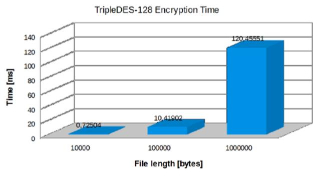
Fig. 18 TripleDES-128 Encryption time
