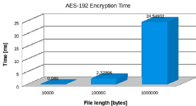
Fig. 21 AES-192 Encryption time
