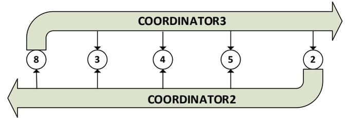
Fig. 3. The case when process 2 receives the  $COORDINATOR_3$  message with a higher ID.
