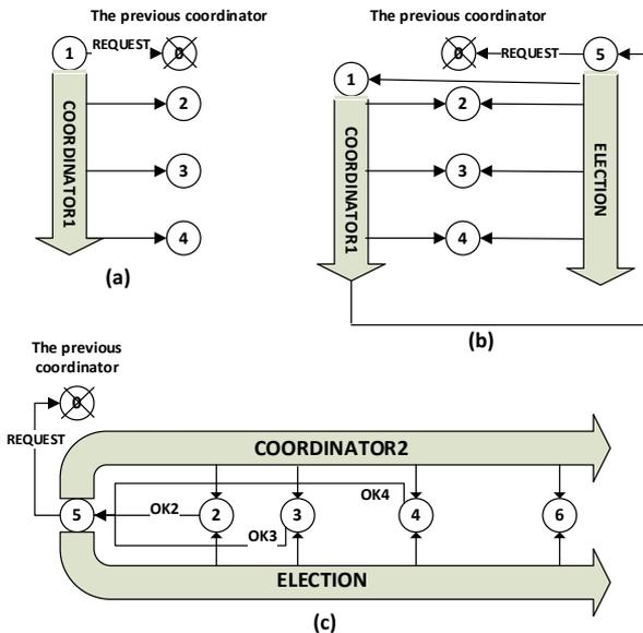
Fig. 1. Electing the new coordinator in case of failure of the previous coordinator: (a) The case when the process with the second minimum ID detects the failure of the coordinator, (b) The case when the process with the second minimum ID receives the  $ELECTION$  message and sends a  $COORDINATOR_i$  message, (c) The case when process 5 selects the new coordinator.
