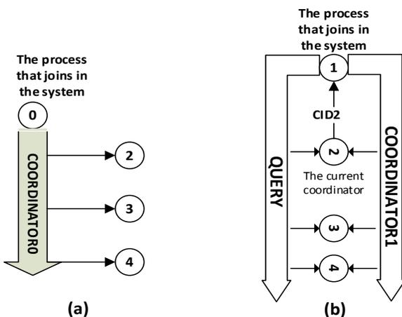
Fig. 2. The case when a new process joins the system: (a) The case when it has the minimum ID, (b) The case when it has a smaller ID than the current coordinator.
