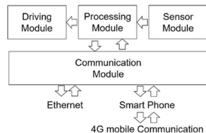
Fig. 5 The block diagram of the embedded system
