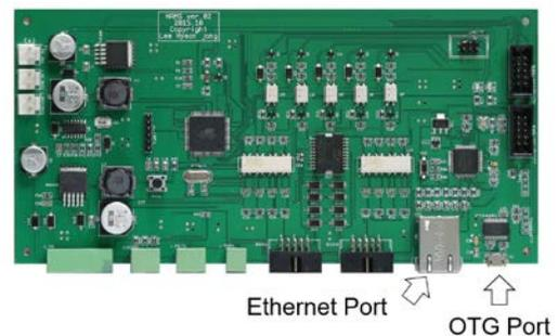
Fig. 6 Developed PCB of the embedded system
