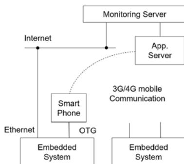
Fig. 2 The overview of multi-channel housing monitoring system
