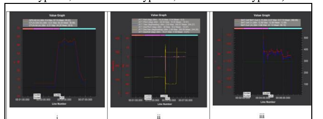
FIGURE 3 – Graphical representation of quadcopter dynamics for single waypoint mission (i- Altitude hold; ii- Pitch, roll & yaw movements; iii- Battery parameters)
