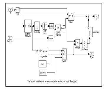
Fig. 3: Arc model simulation block [10].
