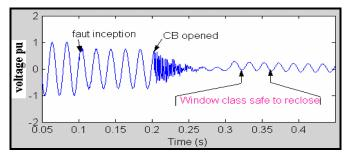
Fig. 6: Transient fault with window from class 2.
