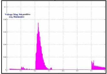
Fig 8: Voltage magnitudes of 9th positive-seq. harmonics.
