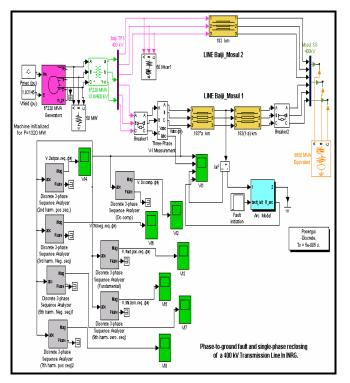
Fig. 2: Simulated Model of Mosul SG-Baijie.
