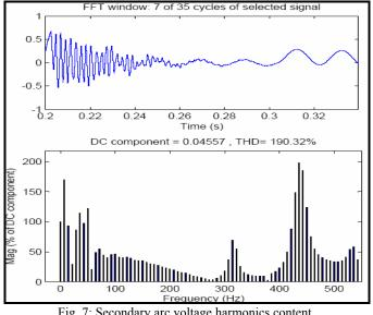
Fig. 7: Secondary arc voltage harmonics content.
