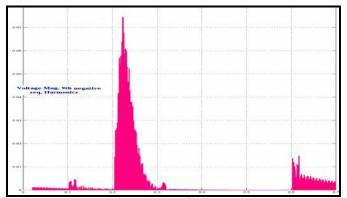
Fig. 9: Voltage magnitudes of 9th negative-seq. harmonics.
