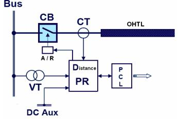
fig. 1: configuration of Transmission Line Bay in HV S/S.
