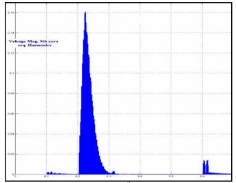
Fig. 10: Voltage magnitudes of 9<sup>th</sup> zero-sequence harmonics
