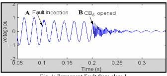
Fig. 4: Permanent Fault from class 1.
