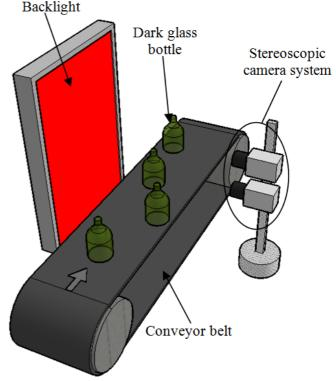
Fig. 2: Scheme of the complete system design.
