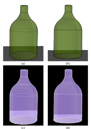
Fig. 3: Detail of the Image Treatment for fast 3D localization. (a) and (b) corresponds respectively to the up (reference) and down simultaneously captured images. (c) and (d) present the foreground extraction result from the images (a) and (b).
