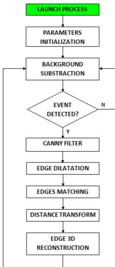
Fig. 6: Chart of the fast 3D localization method.
