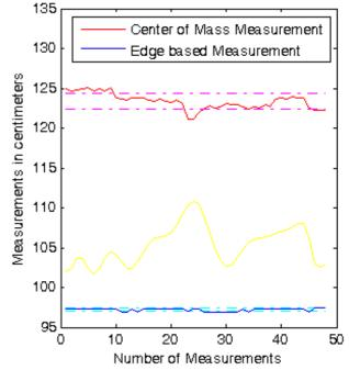
Fig. 10: Positioning error of the center-of-mass (red line) compared with the edge based 3D localization center-of-mass (blue line). The yellow line present some positioning variation along the Y axes to cover the whole image. The magenta dash dot line present the standard deviation centered on average value of red line. The cyan dash dot line present the standard deviation centered on average value of blue line.
