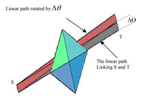
Fig.2 the Interference between the linear trajectory and the obstacle in 3D environment : linear path
