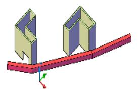
Fig. 7 Free smoothed path realization the insertion of two control points : linear trajectory (Isomertic view)
