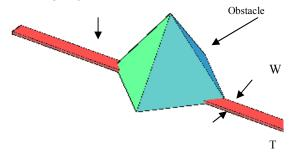
Fig. 1 the Interference between the linear trajectory and the obstacle in 3D environment - isometric view –
