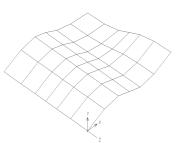
Fig. 16 Mesh creation and 3D surface smoothing: case of Quadratic smoothed B-spline surface
