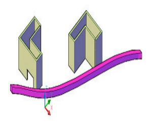
Fig. 8 Free smoothed path realization the insertion of two control points : smoothed path ( Isomertic view)
