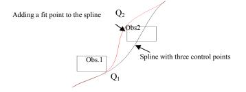
Fig. 3 Addition of control point to a spline curve
