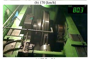
(c) 80 [km/h] Fig. 7 tread braking test at dry condition
