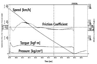
Fig. 15 measurement data under the wet condition at the initial braking speed 200 [km/h]
