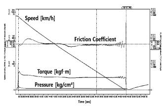
Fig. 14 measurement data under the dry condition at the initial braking speed 200 [km/h]
