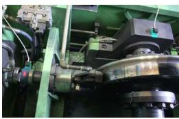
Fig. 6 tread brake blocks of the braking performance tester
