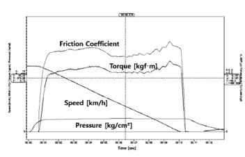
Fig. 9 measurement data under the wet condition at the initial braking speed 80 [km/h]
