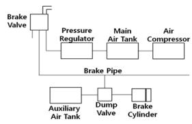
Fig. 1 skeleton diagram of an automatic air brake system
