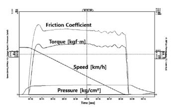
Fig. 8 measurement data under the dry condition at the initial brake speed 80 [km/h]
