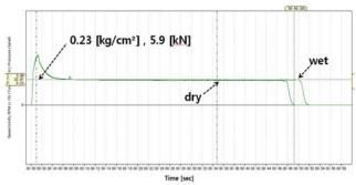
Fig. 18 mutual comparison of pressure in brake cylinder between dry and wet at the initial braking speed 80 [km/h]
