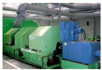
Fig. 4 brake performance dynamometer for high speed train
