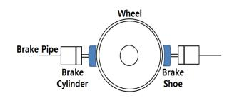
Fig. 2 wheel-tread brake system
