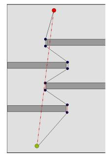
Fig. 6 Trajectory generated using PointBug algorithm in simple maze like type environment.
