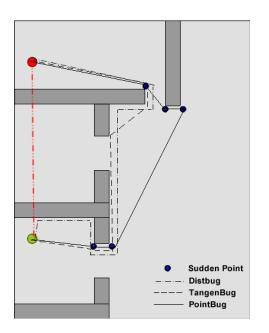
Fig. 8 Trajectory generated using Distbug, TangenBug and PointBugalgorithm in simple Office like Environment.
