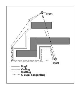
Fig. 2 Trajectories generated by a few bug algorithms
