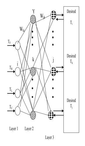
Fig. 4 Target Localization Neural Network
