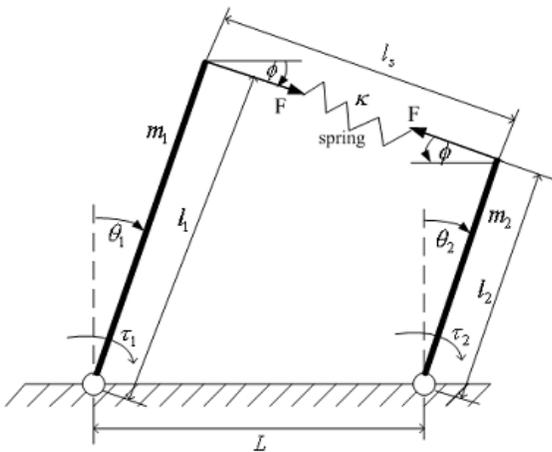
Fig 1. Two inverted pendulum coupled by spring
