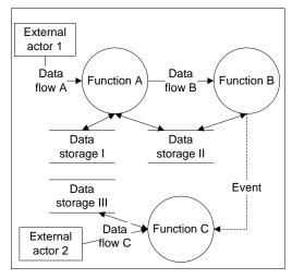
Fig. 3 data flow diagram as a tool of data modeling
