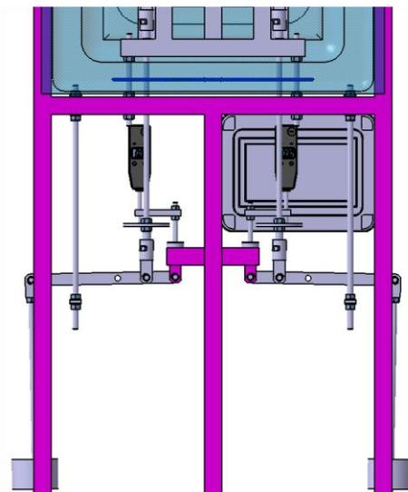
Fig. 7 Lever mechanism
