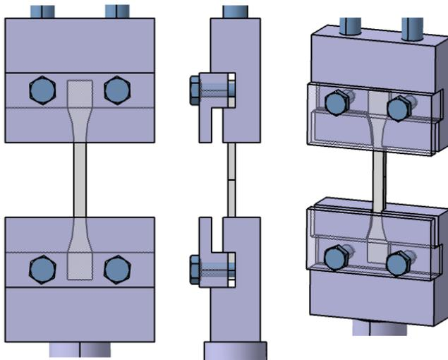
Fig. 2 Clamping of the sample
