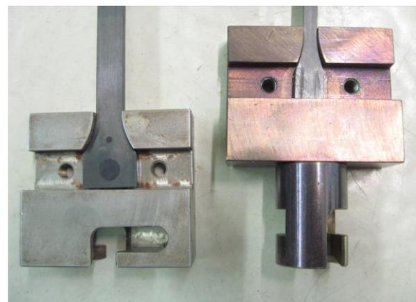
Fig. 4 Comparison of mechanisms for fast loading
