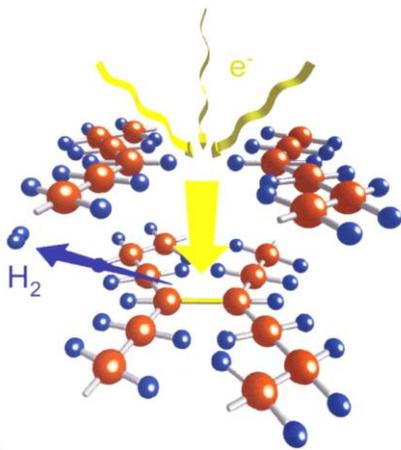
Fig. 17 Principle of radiation crosslinking [1]
