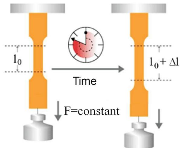
Fig.1 Creep test under a constant load
