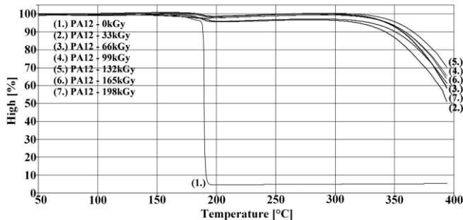
Fig. 14 PA12 thermomechanical analysis
