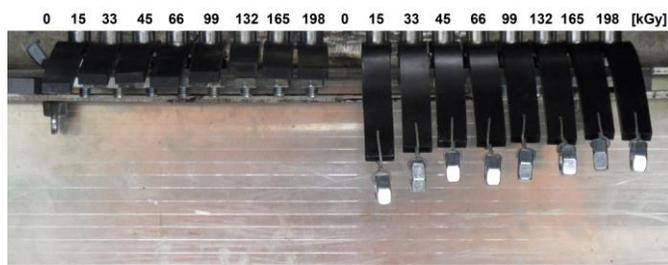
Fig. 19 PA6 specimen deformation after 2 hours temperature exposure 250°C
