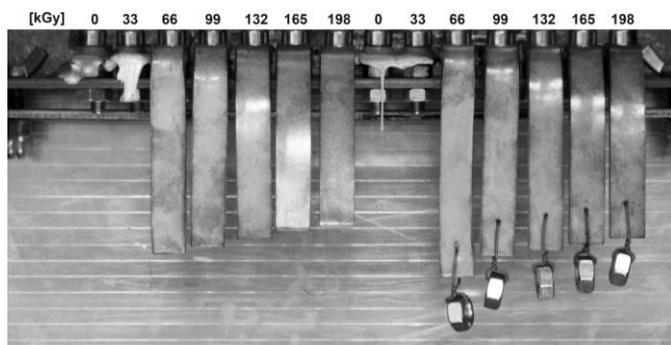
Fig. 13 PBT specimen deformation after 2 hours temperature exposure 250°C
