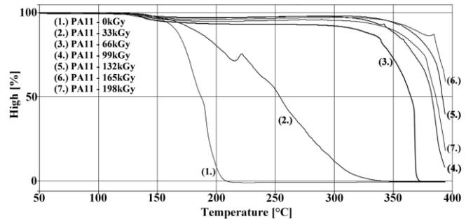
Fig. 16 PA11 thermomechanical analysis
