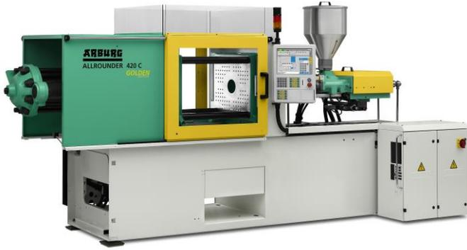
Fig. 4 Injection molding machine ARBURG Allrounder 420C [3]
