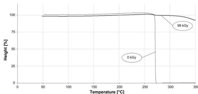
Fig. 20 PA66 thermomechanical analysis
