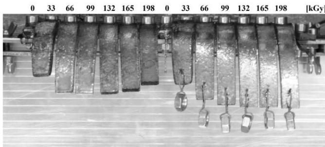
Fig. 7 LDPE specimen deformation after 2 hours temperature exposure 220°C
