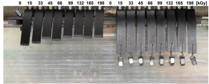
Fig. 21 PA66 specimen deformation after 2 hours temperature exposure 300°C
