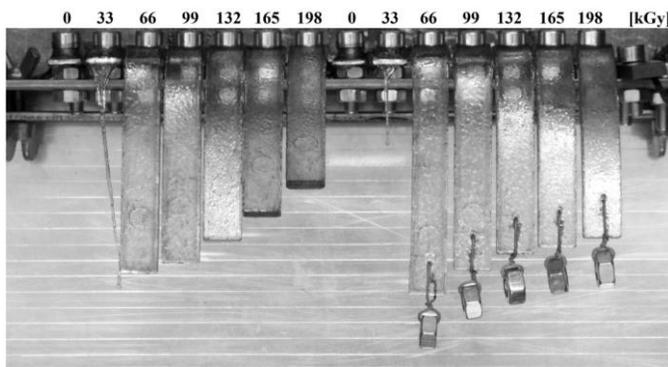
Fig. 9 HDPE specimen deformation after 2 hours temperature exposure 220°C
