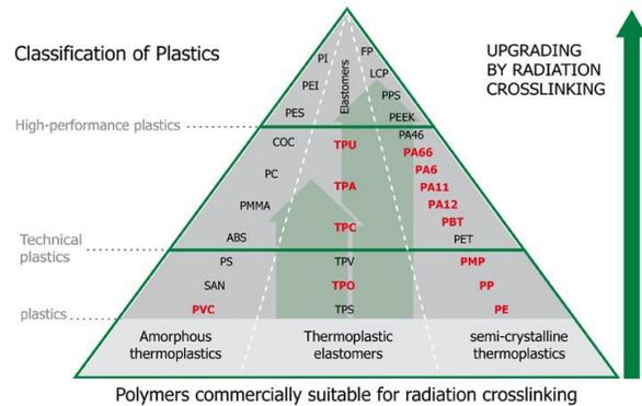
Fig. 3 Pyramid of Polymers [2]
