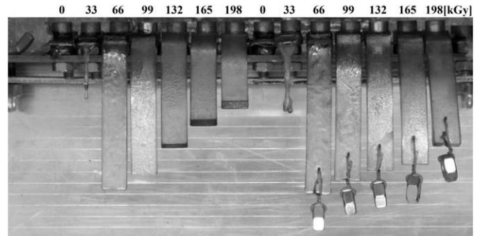
Fig. 11 TPE specimen deformation after 2 hours temperature exposure 220°C
