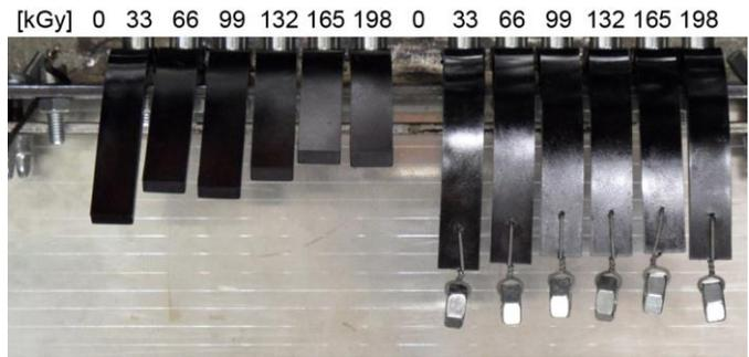
Fig. 15 PA12 specimen deformation after 2 hours temperature exposure 250°C
