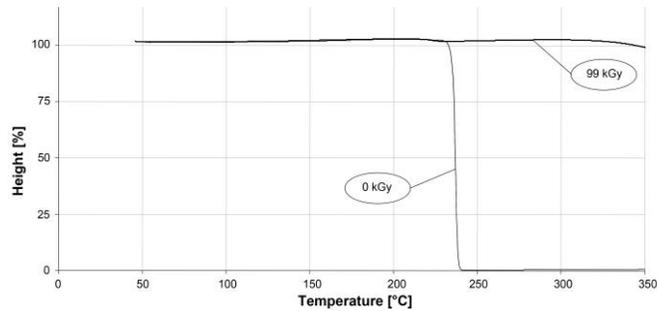
Fig. 18 PA6 thermomechanical analysis
