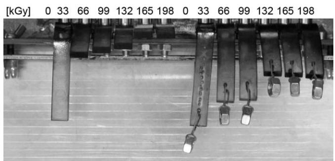
Fig. 17 PA11 specimen deformation after 2 hours temperature exposure 250°C
