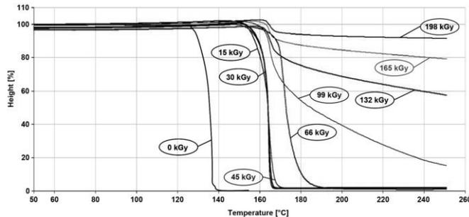
Fig. 8 HDPE thermomechanical analysis
