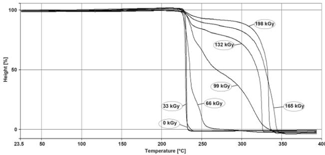
Fig. 12 PBT thermomechanical analysis
