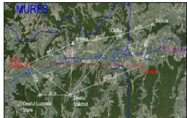
Fig. 5. Points in the National Geodetic Network along the C.F. Sighișoara-Ațel section
