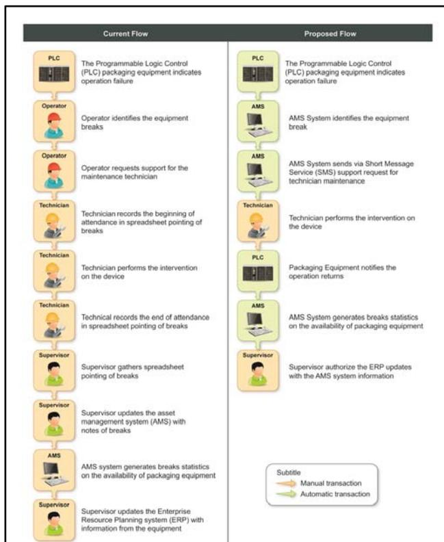
**Fig. 4: Flow of current and proposed corrective maintenance in packaging equipment**
