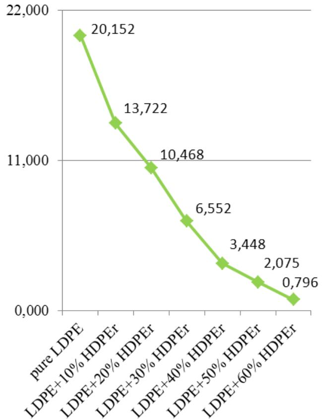
Fig. 9 Mass flow rate
