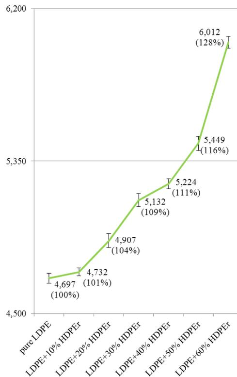
Fig. 15 Ultimate tensile strength
