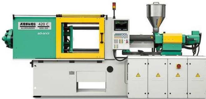
Fig. 8 Injection molding machine
