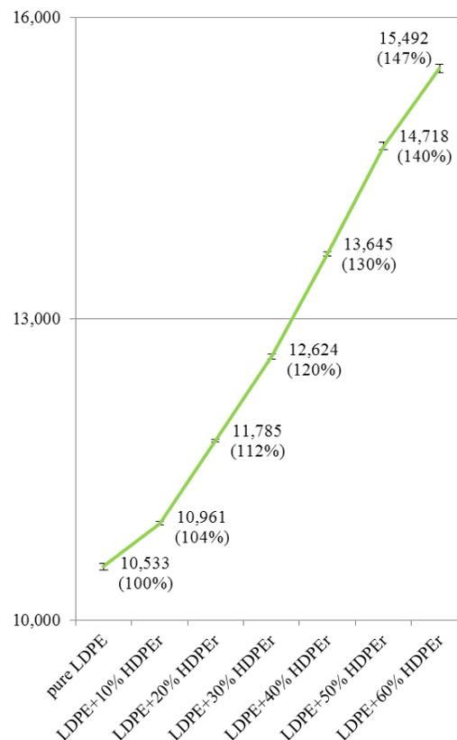
Fig. 12 Ultimate tensile strength
