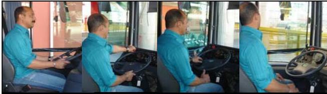
Fig. 3 pictures sequence showing the conductor switching from manual to automatic guidance (Expresso Tiradentes bus corridor – Sao Paulo)
