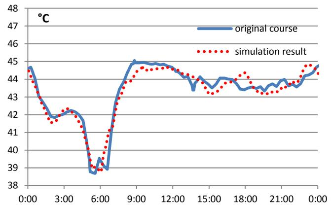
Fig. 14 Water temperature in returning pipe
