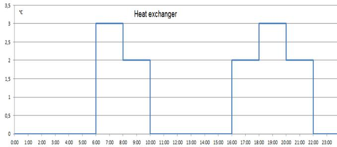
Fig. 16 Proposed changes in the temperature of heating water (heat exchanger stance)
