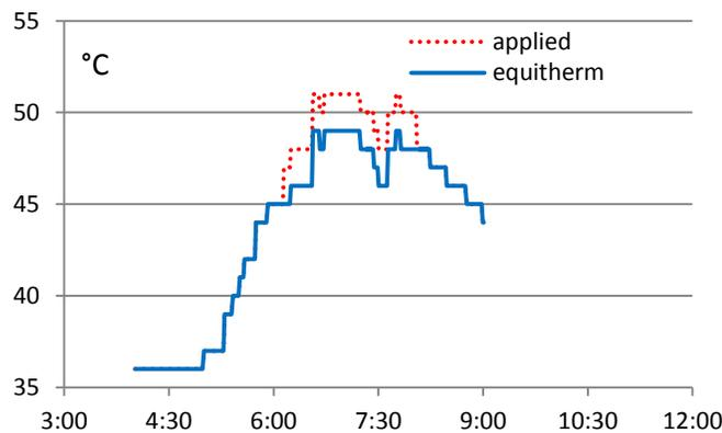
Fig. 18 Applied heating water temperature (house station)
