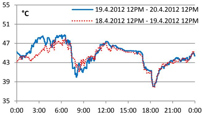
Fig. 26 Water temperature on return (exchanger stance)
