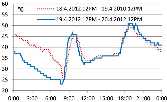
Fig. 21 Heating water temperature (house station)
