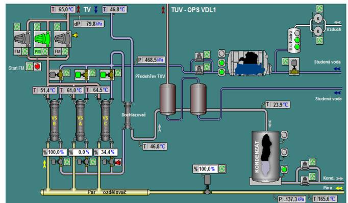
Fig. 6 Heat exchanger stance diagram
