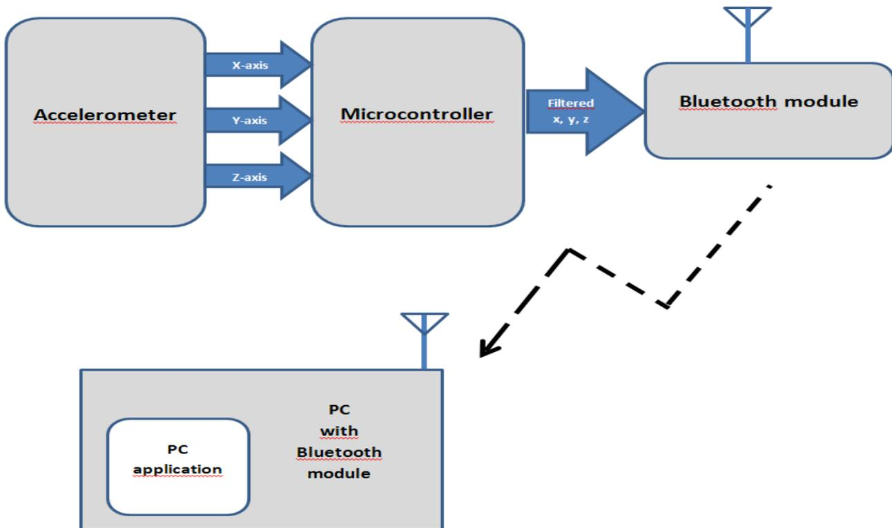
Fig. 4 Block diagram of the system
