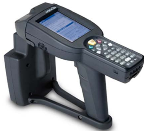
Fig. 3 Merlin UHF RFID Cross Dipoli handheld reader
