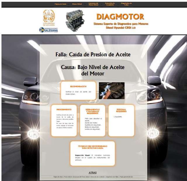
Fig. 11. Example of a Possible Cause in the Troubleshooting section of the Diagnosis ES.
