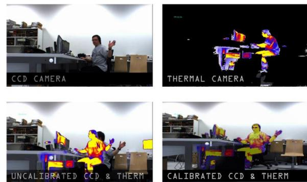
Fig. 24 image of CCD camera (upper left), image of thermal imager (upper right), uncalibrated data fusion (bottom left), calibrated data fusion (bottom right)
