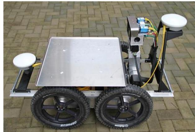
Fig. 4 Orpheus-X4 robot with sensor head and landing area for multicopters
