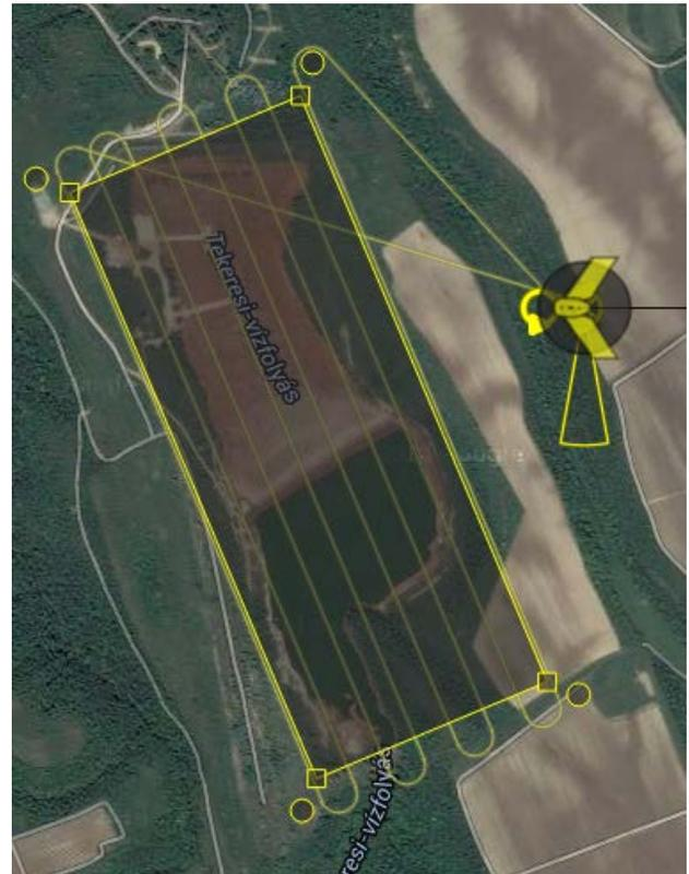
Figure 4: Autonomous mission plan in "Sensefly eMotion 2"
