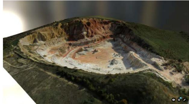
Fig. 15: Reconstructed quarry textured model
