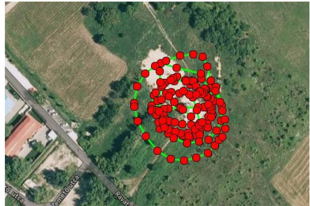
Fig. 11: The position of the basic picture of the chapel (Pix4Dmapper)
