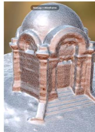
Fig. 14: 3D reconstructed object ("chapel") visible object faces - Sketchfab
