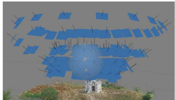
Fig. 12: The position and orientation of the raw images of the chapel (Agisoft Photoscan)
