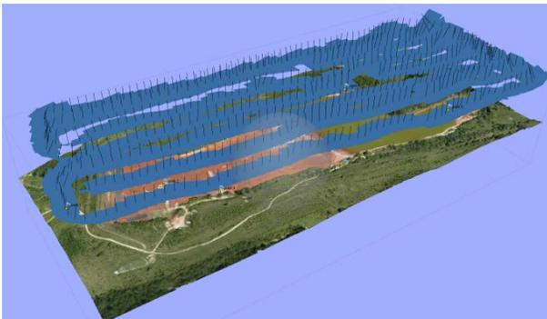
Fig. 3: The spatial positions and orientations of the images of the surveyed area (Agisoft Photoscan)
