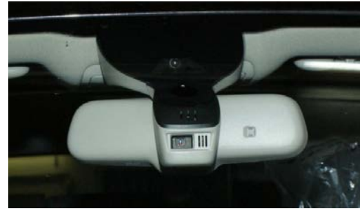
Fig. 2. Placement of sensor-module in cars. Sensors of module (from top to bottom): lane keeping system camera, rain and light sensor, adaptive lighting system camera [12].
