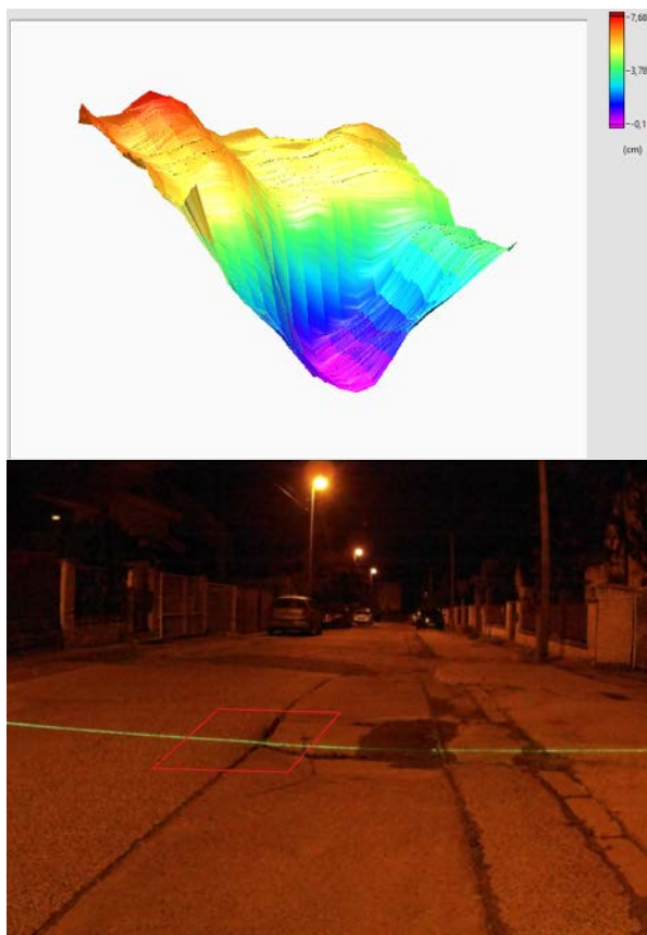
Fig. 7. Generated surface map (above) and characteristic instance of source image set (below) with mapped area marked (red).
