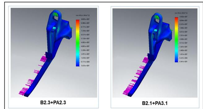
Fig. 9 Example of lateral test simulation
