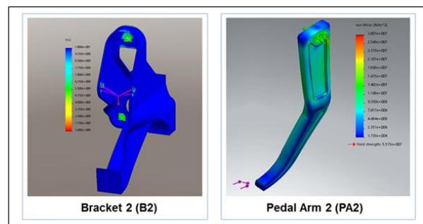
Fig. 7 Example of the simulation analysis using Aluminium Alloy 6061
