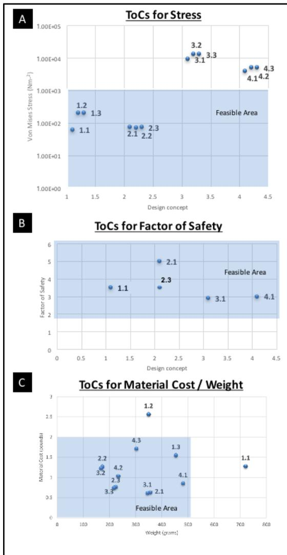
Fig. 8 Example of ToCs for bracket
