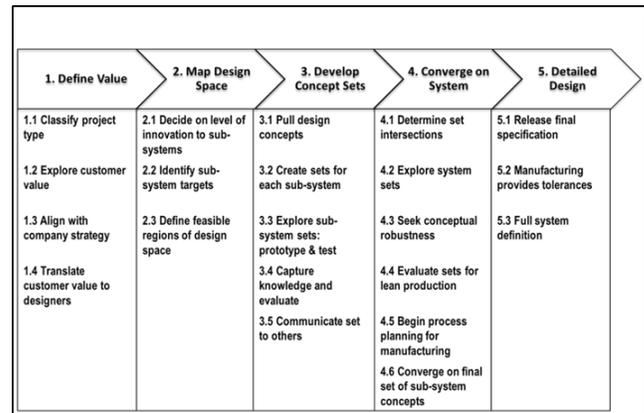
Fig. 2 The SBCE process model
