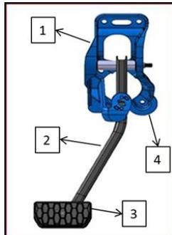
Fig. 4 The system level of brake pedal box
