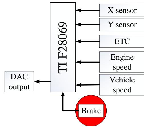
Fig. 6 The structure of clutch control experiment
