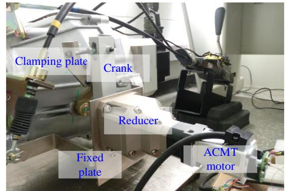
Fig. 12 Illustration of ACMT actuator
