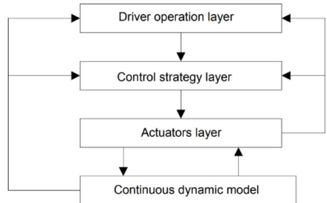
Fig. 1 The controller signal flowchart of ACMT
