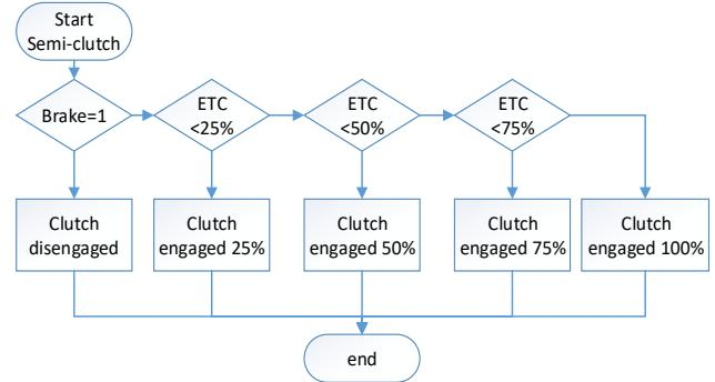
Fig. 5 Semi-clutch logic flow chart
