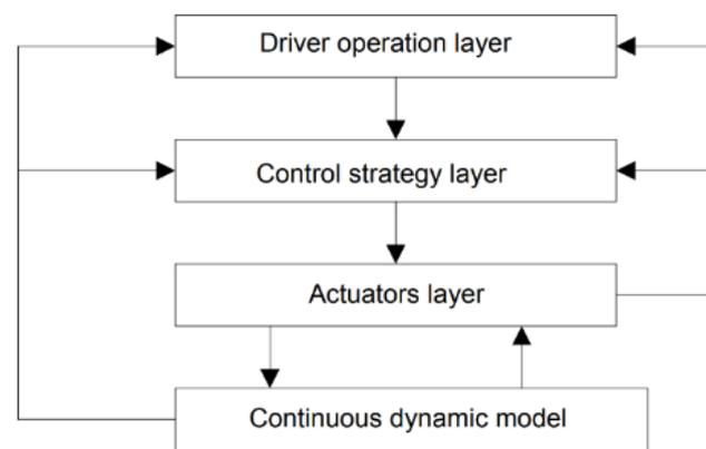
Fig. 1 The controller signal flowchart of ACMT
