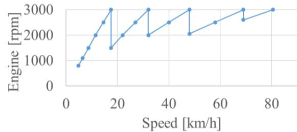
Fig. 7 Definition of upshift engine speed
