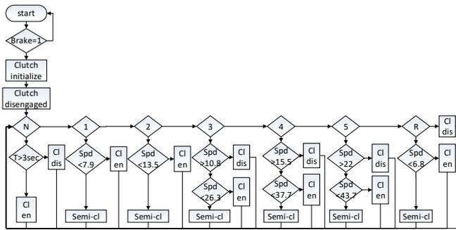
Fig. 2. ACMT control logic flow
