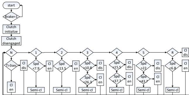
Fig. 2. ACMT control logic flow
