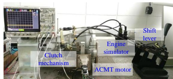
Fig. 11 Photograph of ACMT test platform
