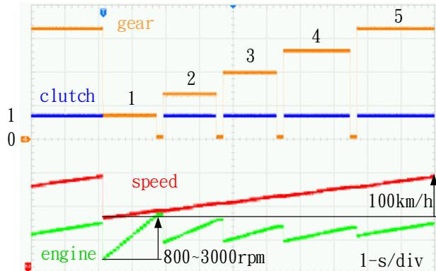
Fig. 2 Upshift speed clutch position result
