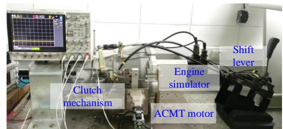
Fig. 11 Photograph of ACMT test platform
