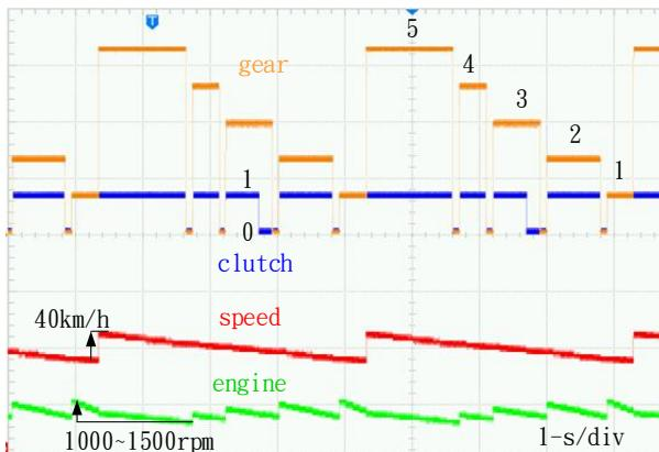
Fig. 10 Downshift speed clutch position result
