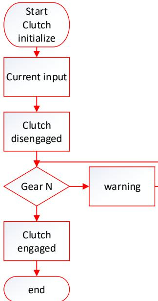
Fig. 3 The initialization of the clutch position control
