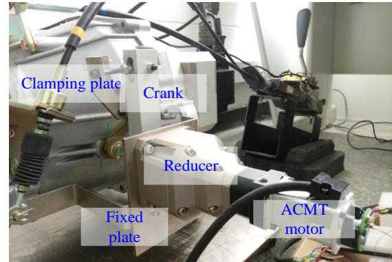
Fig. 12 Illustration of ACMT actuator
