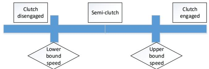
Fig. 4 Three categories of the clutch position: fully engaged, semi-clutch and disengaged according to different speeds
