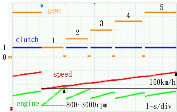
Fig. 2 Upshift speed clutch position result
