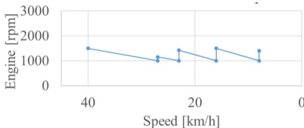
Fig. 9 Definition of downshift engine speed
