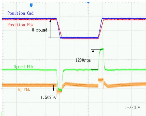
Fig. 3 ACMT clutch control performance
