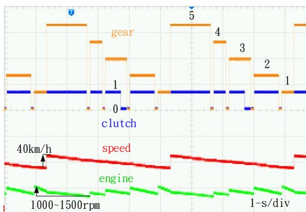
Fig. 10 Downshift speed clutch position result
