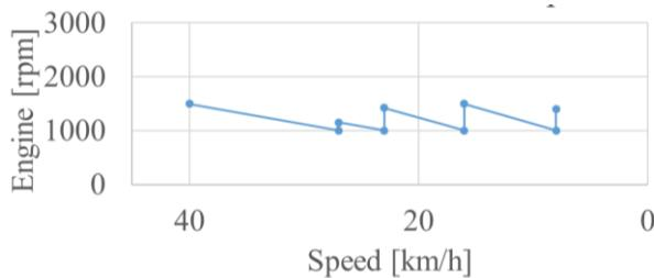
Fig. 9 Definition of downshift engine speed
