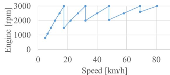
Fig. 7 Definition of upshift engine speed
