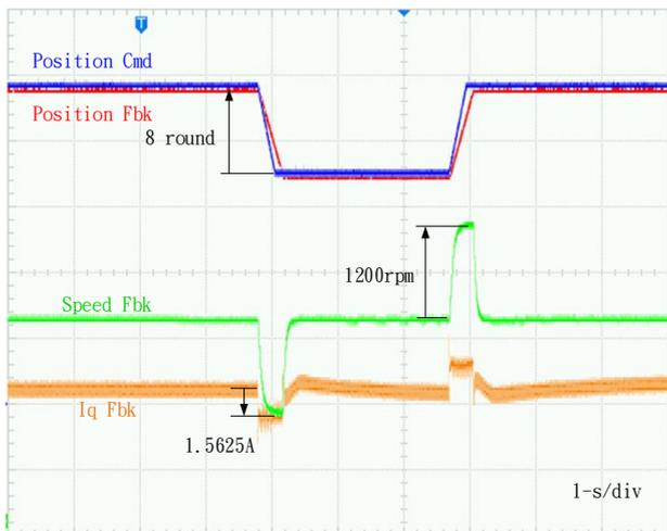
Fig. 3 ACMT clutch control performance
