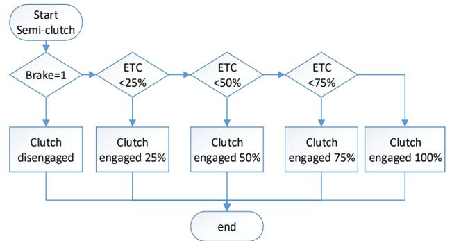
Fig. 5 Semi-clutch logic flow chart
