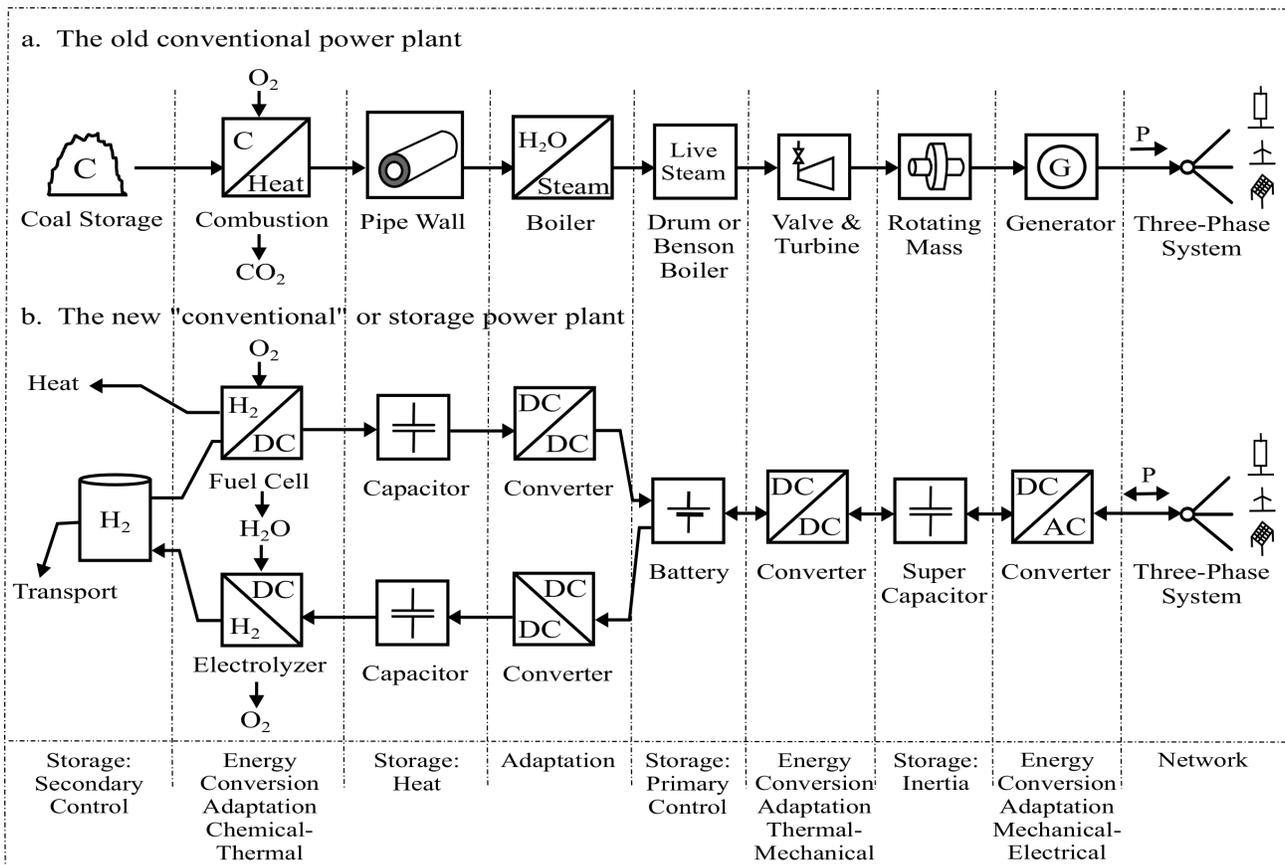
Fig. 1. Comparison between the (a) existing fossil fuel based and (b) new storage power plant
