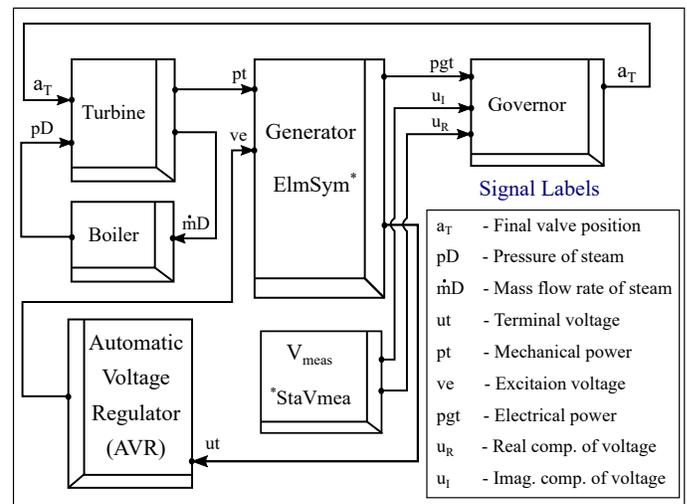
Fig. 5. Composite model for the synchronous generator representing a thermal power plant governed by angle control
