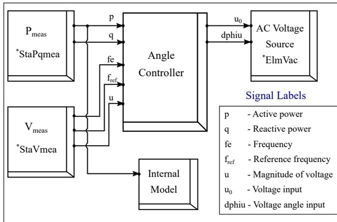
Fig. 3. Composite model for the AC Voltage Source representing a storage power plant
