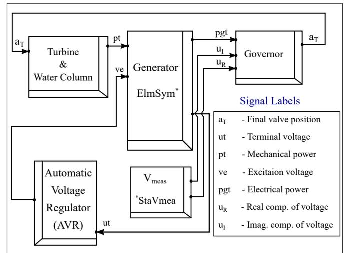
Fig. 6. Composite model for the synchronous generator representing a hydro power plant governed by angle control
