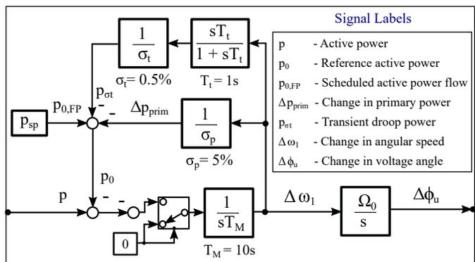
Fig. 4. Common model for the angle controller of the slack storage power plant
