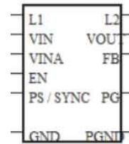
Fig.3 TPS63020 pin diagram
