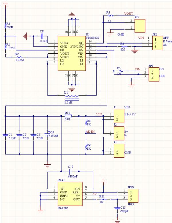
Fig.4 DC-DC conversion circuit schematic
