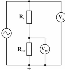
Figure 3 Passive test circuits ( $R_x$  symbolizes the measured Debye model circuit)
