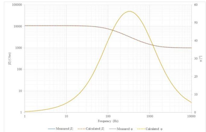
Figure 4 Result of EIS measurement performed on a test circuit compared to the theoretical values
