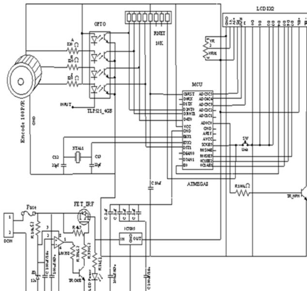
Fig. 2. The contact tachometer circuit
