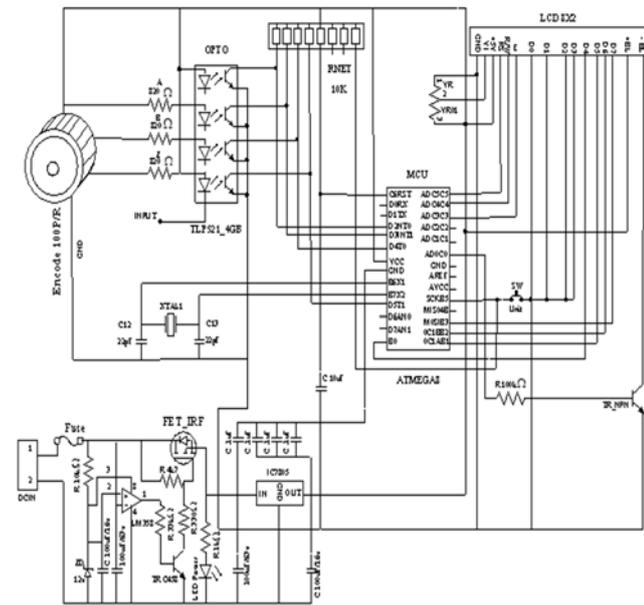
Fig. 2. The contact tachometer circuit
