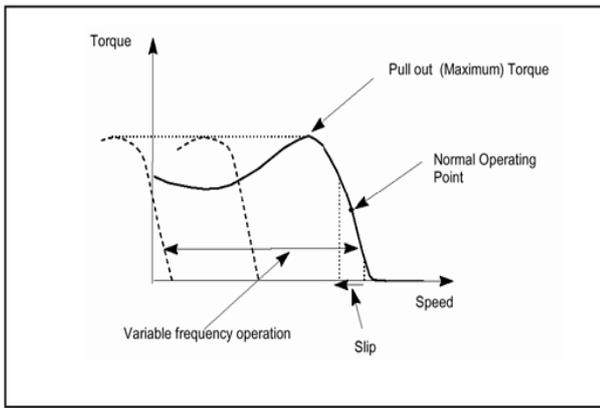
Fig. 1. Characteristics of torque to the speed of AC motors.
