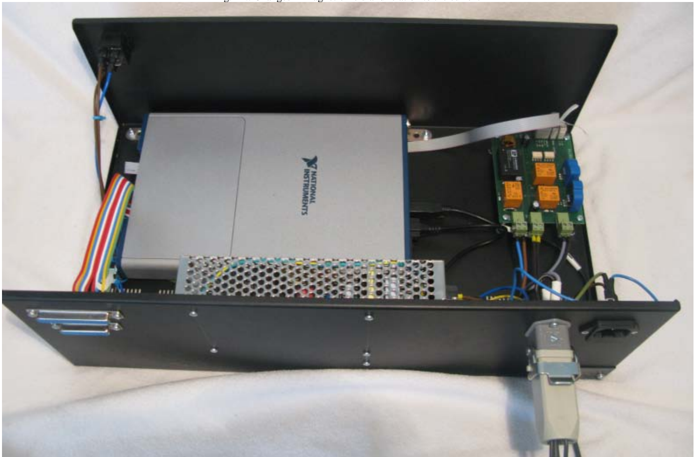
Fig. 13.: Completed device used for FFT / Air load tests
