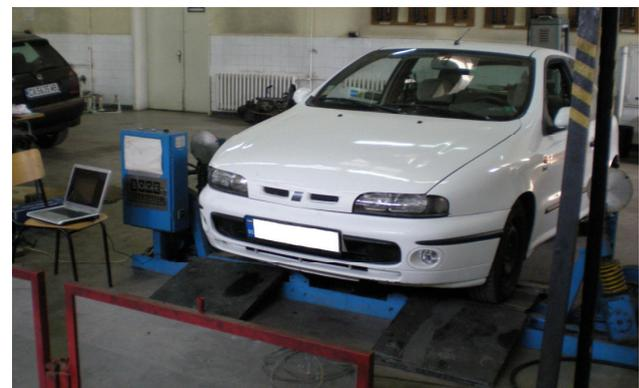
Fig. 2. Vehicle situation on the vibration stand
