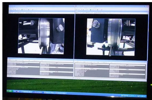
(c) Wheel/rail contact monitoring at the control station
