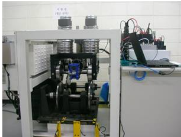
Fig.18 Scaled roller rig for the load test of the driving motor
