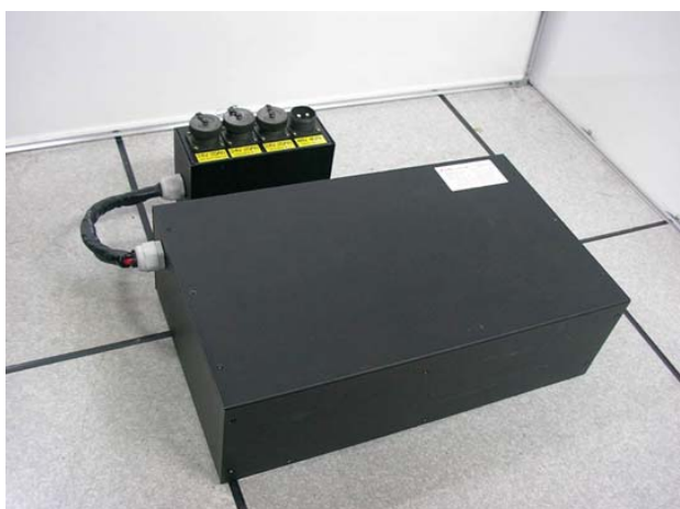
(a) The main battery part for providing a driving motor, two actuators and a controller with power
