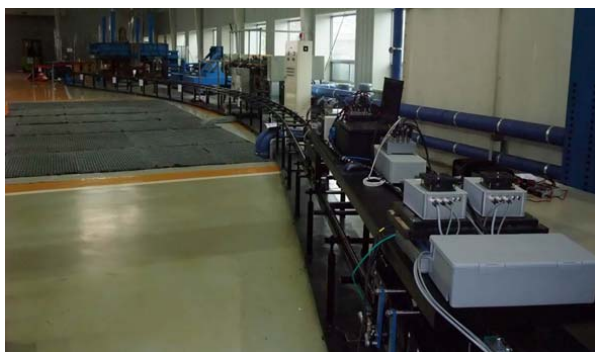
Fig.6 Research testbed: the 1/5 scale active steering vehicle and the curved track
