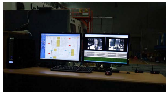
Fig.7 Control station module for remote control and signal monitoring remotely
