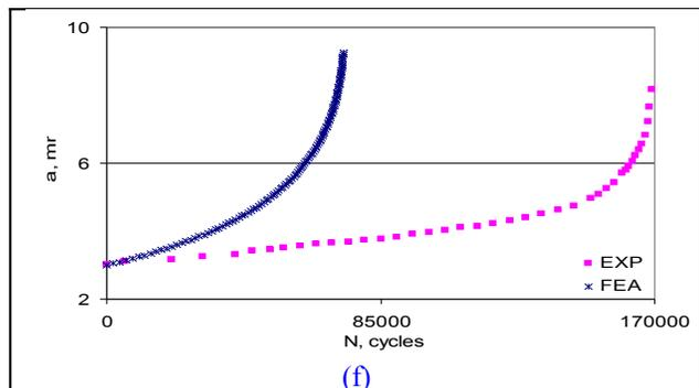
Fig. 6: Experimental and FE results (crack length vs number of cycles at stress levels in % of yield strength). a) 40 b) 35 c) 30 d) 25 e) 20 f) 15.
