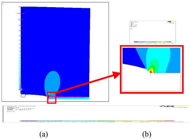
Fig. 4: a) Von Mises stress distribution at stress level of 40% and crack length 4 mm. b) Crack tip region.
