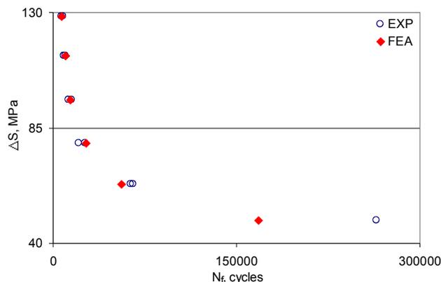
Fig. 7: SN curves: Experimental vs FEA.
