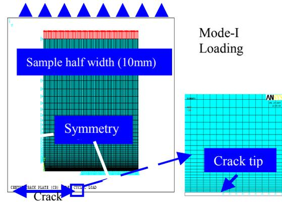
Fig. 3: a) Quarter model of the MT sample - element plot with applied boundary conditions, b) Crack tip region showing mapped meshing.
