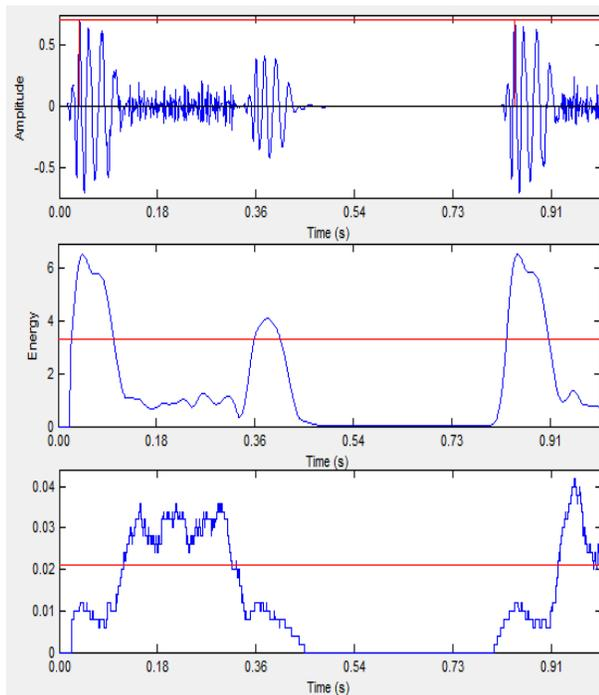
Fig. 10 Cardiac signal with systolic murmur and its associated *RMS* and *ZCR*.
