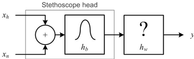
Fig. 4 Filtering scheme for noise reduction at stethoscope head level.
