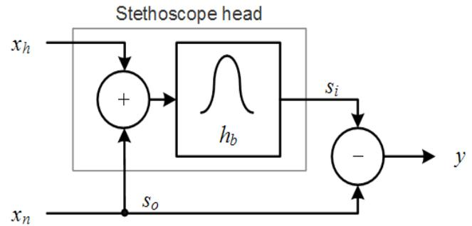
Fig. 6 Direct difference method for noise reduction.
