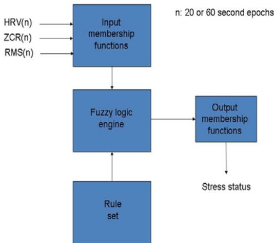
Fig. 12 Fuzzy-logic decision engine to decide about the behavioural state (stress level) of a subject from data detected by PCG and ECG subsystems.
