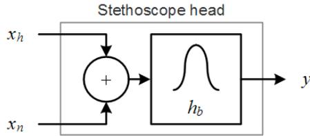
Fig. 3 Signal and noise add and convolution in the head of a traditional stethoscope.
