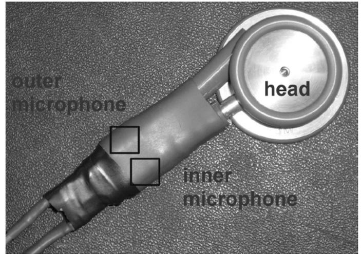
Fig. 5 Double microphones modified head stethoscope.
