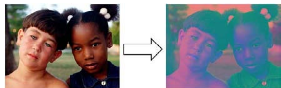
Fig. 4 Transformation from RGB to YCbCr color model
