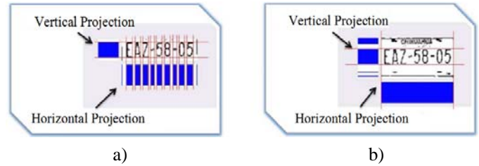
Fig. 11 vertical and horizontal projections. a) from the ROI detected by match and b) from the ROI detected by rectangles.
