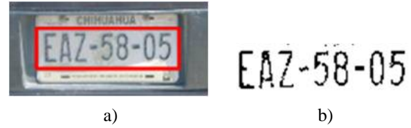
Fig. 10 a) ROIs detected and b) the result of thresholding the ROIs detected.
