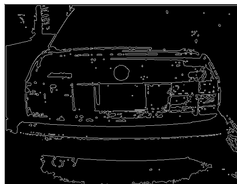
Fig. 5 image obtained with Canny filter.
