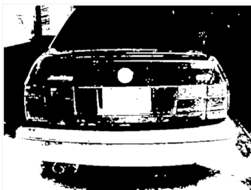
Fig. 4 resulting image after dilate-erode.
